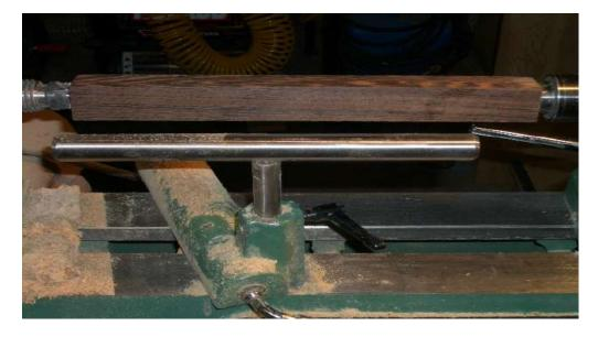
When turned, it seemed to me that the handle was feeling a bit narrow in my hand. So I decided to add some thickness on one end by adding a piece of birds eye maple. I thought the contrasting wood would make an interesting feature. To do this I made sure the end to receive the maple was exactly 3/4 inch in diameter for about 4 inches of length. Then, on a drill press, I drilled a 3/4 inch hole through the birds eye maple and subsequently epoxied it onto the wenge shaft.
