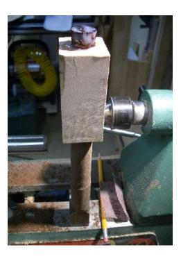
After curing the assembly was mounted between centres and the square end turned to exactly 1/2 inch. This assembly was then mounted into a 1/2 inch collet chuck and turned to final shape. Sanding to 400 grit was carried out and the handle set aside until it was to be epoxied into the head.
