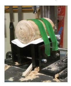
When the hole was done, the head was completed by manually removing the leftovers of the tenons from both faces (crowned ends). A carving knife was used for the majority of the rough work. Then a sanding pad in a Jacob chuck was installed in the Morse taper of the headstock. This made the process much easier because I
