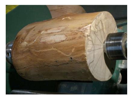
I turned it round, marked out the transitions, turned the rough shape and marked centre for the handle hole. I then selected where I wanted to place the handle and, using an awl marked a point on the line that would survive sanding efforts.
